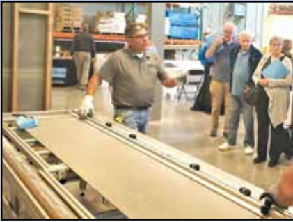
2018 recap: IMI tile apprentice instructor Dan Cosgrove demonstrated the handling and cutting of a 10-foot panel of thin gauged porcelain tile for a group of architects and contractors at the 2018 Chicago TMT Expo.
